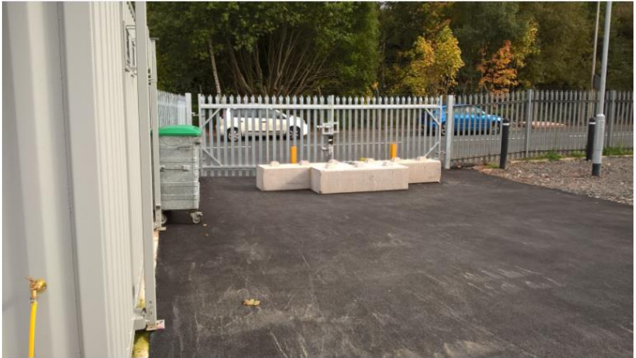
Entry gate with movable security concrete blocks and removable posts (in yellow)
