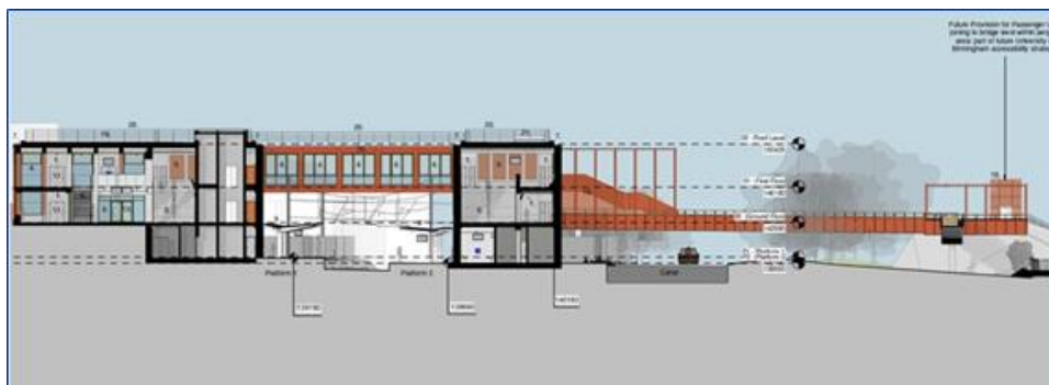
GRIP 4 Section Through Proposed New Station Building. Source: University Station Planning Application Documents, November 2019
