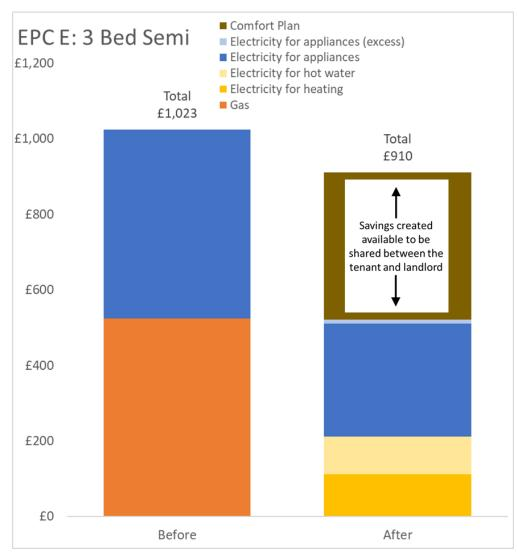
The total annual energy bill for the tenant for gas and electricity is estimated at  $\pm 1,023$ . After the Energiesprong whole house retrofit, upgrading the property to EPC A the total energy bill for heating, water and appliances is projected to drop to around  $\pm 503 - a$  saving of  $\pm 520$  p.a. or reduction of 50%.
