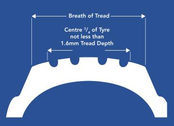
Most car tyres have tread wear indicators, these are small ribs across the main tread grooves, and when the tread surface becomes level with these ribs the tyre is at the legal limit and must be replaced.
