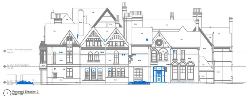
Image 2 – Proposed elevation showing the new external staircase and openings for externally accessible toilets (side elevation and rear courtyard)
