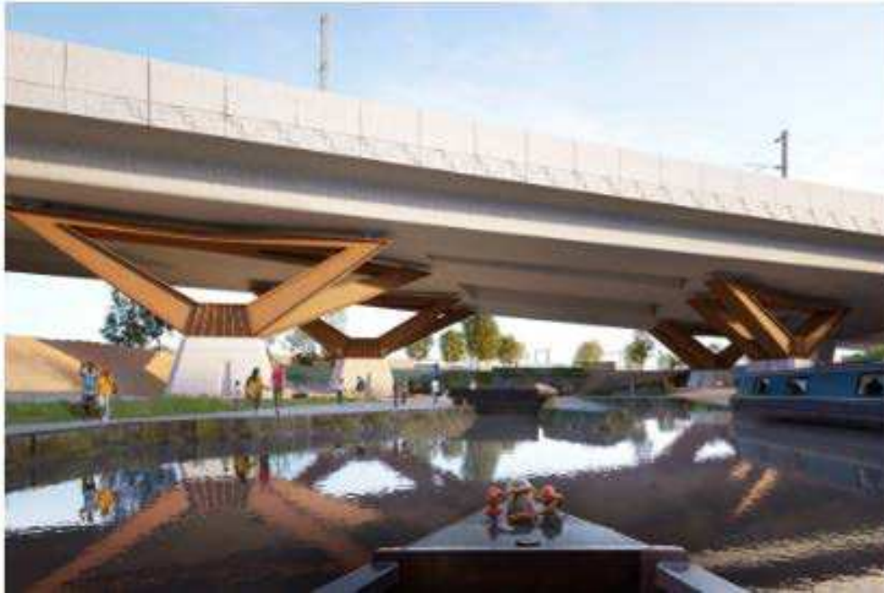
Fig 6. CGI of the bespoke tripod piers over the canal and coffers viewed from underneath. Please note that public realm works beneath the canal are proposed to come forward at a future stage and are not the subject of this application submission.
