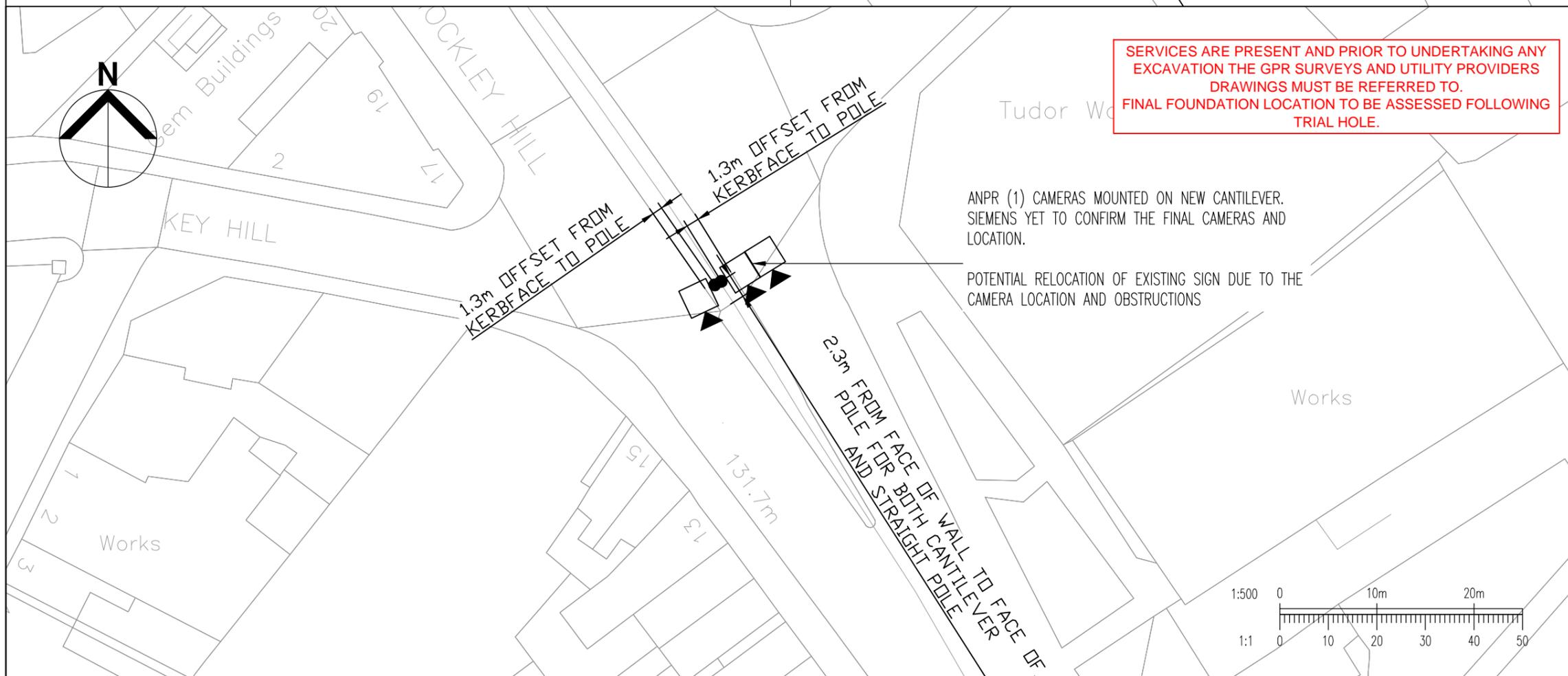
SERVICES ARE PRESENT AND PRIOR TO UNDERTAKING ANY EXCAVATION THE GPR SURVEYS AND UTILITY PROVIDERS DRAWINGS MUST BE REFERRED TO. FINAL FOUNDATION LOCATION TO BE ASSESSED FOLLOWING TRIAL HOLE.
