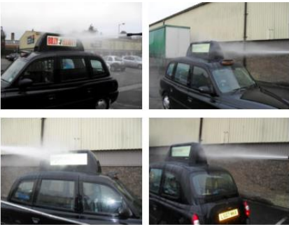
The installed unit was subjected to water jet testing at 120 Bars from a distance of 2M from six different axes. The unit was powered up and continuously on throughout the test.
