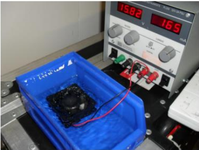
The installed unit was subjected to water jet testing at 120 Bars from a distance of 2M from six different axes. The unit was powered up and continuously on throughout the test.
