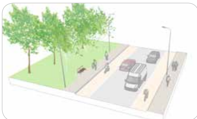
Indicative section of the reconfigured urban street at the eastern edge of the ring road, where existing road space can be reorganised to accommodate cycle lanes
