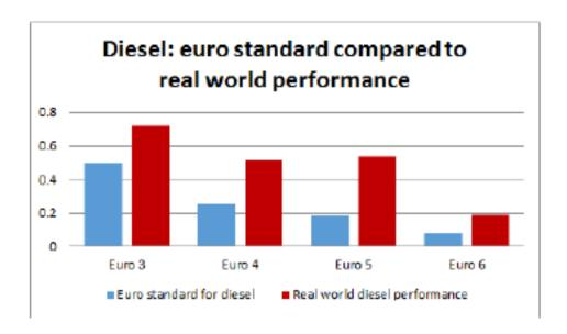
6.12 As may be seen, petrol cars are performing within the Euro standard whereas diesel cars, of which there are an increasing number are not. This is why the CAZ approach (see below) focuses more on diesel vehicles than petrol.
