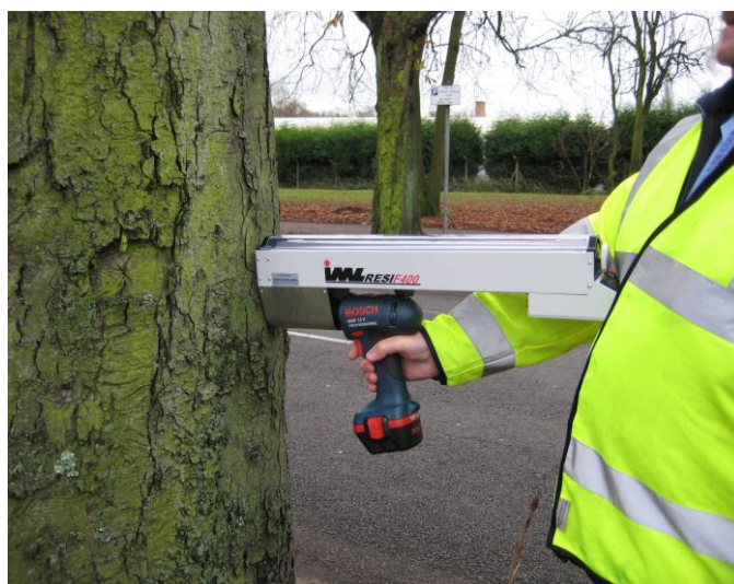
Resistograph Decay Detection
